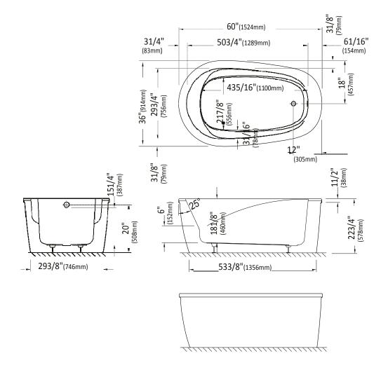
\* A bathtub fitted with back jets can cause the pump to protrude by approximately 3" from the overall dimension.
