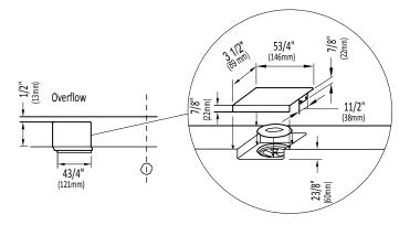
\* A bathtub fitted with back jets can cause the pump to protrude by approximately 3" from the overall dimension.
