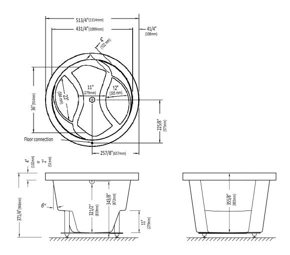
\* A bathtub fitted with back jets can cause the pump to protrude by approximately 3" from the overall dimension.
