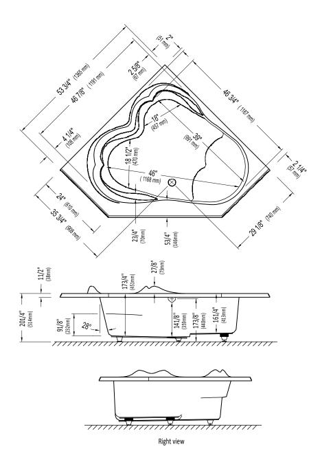
\* A bathtub fitted with back jets can cause the pump to protrude by approximately 3" from the overall dimension.
