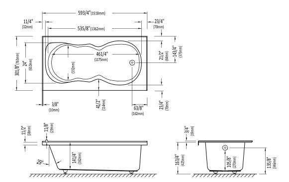
\* A bathtub fitted with back jets can cause the pump to protrude by approximately 3" from the overall dimension.
