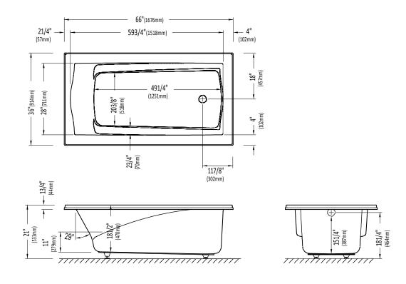
\* A bathtub fitted with back jets can cause the pump to protrude by approximately 3" from the overall dimension.
