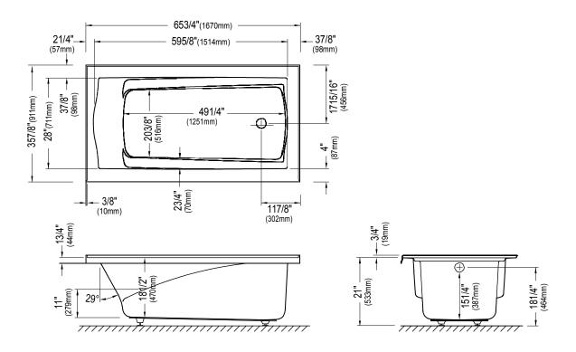
\* A bathtub fitted with back jets can cause the pump to protrude by approximately 3" from the overall dimension.
