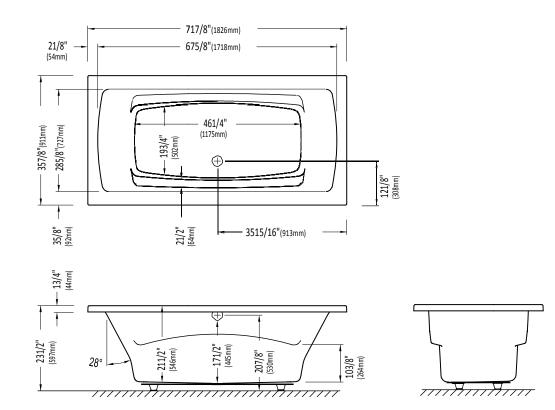
\*A bathtub fitted with back jets can cause the pump to protrude by approximately 3" from the overall dimension.
